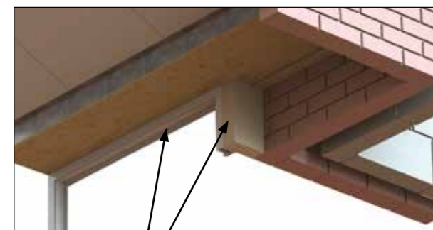
Existing frames and infill
